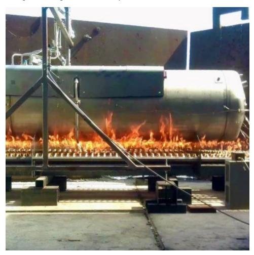
The liquid hydrogen tank system for trucks developed by Austrian company SAG has reached a decisive milestone on the way to approval for road traffic: the successful completion **of the so-called Bonfire test**.
