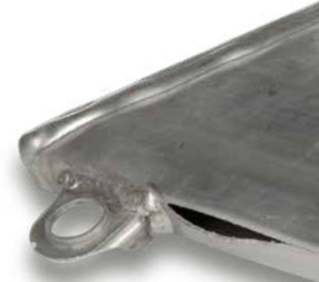
Burst Test Result for Air Tank
