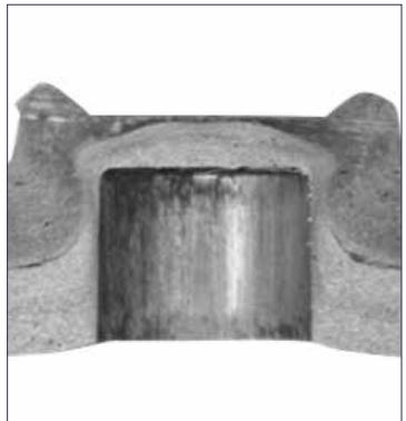
Cross Section through Tox Joint
